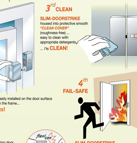
**SLIM-DOORSTRIKE** Automatic fail-safe unlock. In the event of fire or power failure it automatically unlocks freeing the exit... .... it's FAIL-SAFE!
