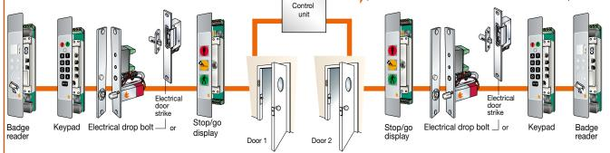
Diagram of the equipment required to configure a door interlocking system with mutual acknowledgment
